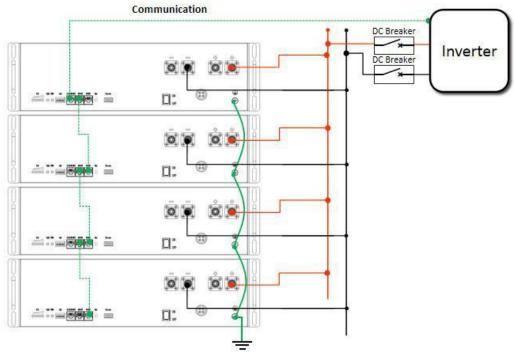
Figure 7 - Multi-Units Connection-2 ( Battery  $\Delta V$  should be less than 3V at first Parallel installation )
