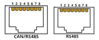
Figure 4 - CAN/RS485 and RS485 connections
