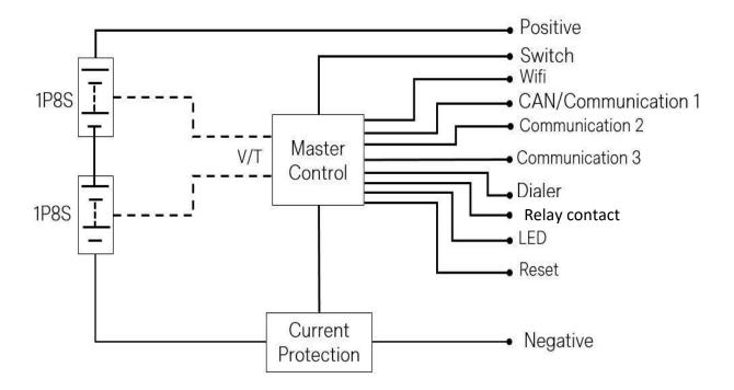
Figure 1 - System Schematics
