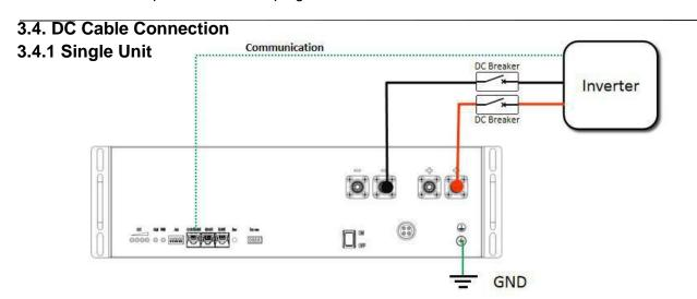
Figure 5 - Single Unit Connection
