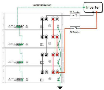
Figure 6 - Multi-Units Connection-1 ( Battery  $\Delta V$  should be less than 3V at first Parallel installation )
